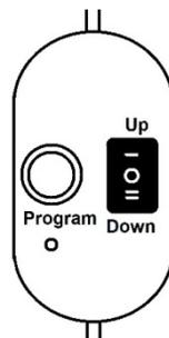
The monostable "Program" button allows for applying voltage to the 'up' direction.
