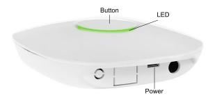
At first use, the button is white (the control unit in direct connection mode - Access Point).
